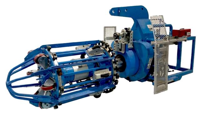
The RMS Counterbore Machine (CBM) is used to machine internal transitions. This allows pipe of unequal wall thickness to be machined and matched.
